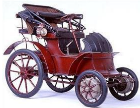
1900 Lohner Porsche car with electric motors integrated into the wheels (Wienkötter, 2018).
