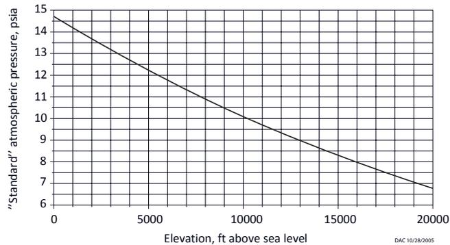
Fig. 12.4. Atmospheric Pressure as a Function of Elevation
