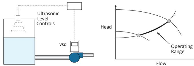
**Fig. 9.10.** Level controls using a vsd equipped pump
