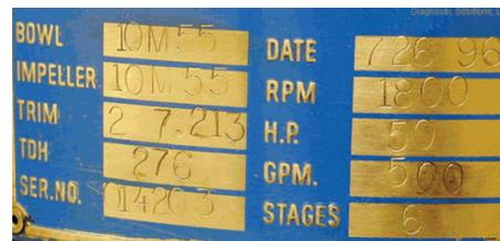
Fig. 12.1. Motor and Pump Nameplate Data
