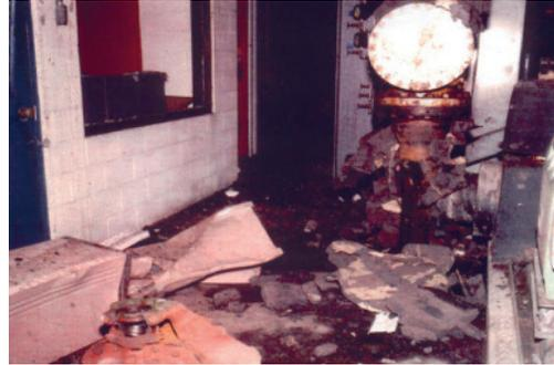
**Fig. 6.2.** Explosion due to closed valves on both sides of a pump
