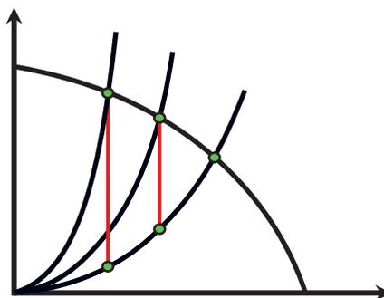
**Fig. 7.4.** Throttling a valve changes the flow rate by adding the pressure drop in the valve to the system losses. The new system curve will be steeper and the operating point moves up along the pump curve.
