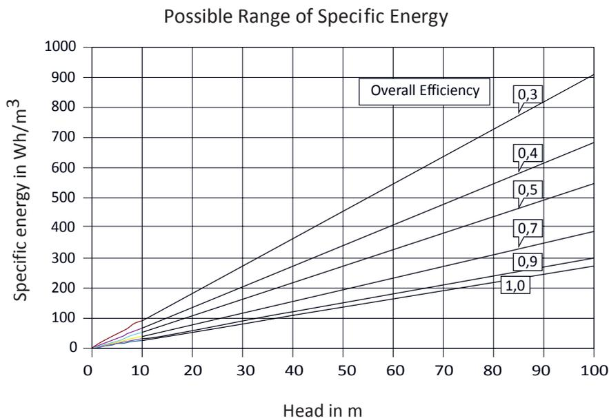
Fig. 7.2. Specific energy as a function of head for different overall efficiencies ( $= \eta_{drive} * \eta_{motor} * \eta_{pump}$ )
