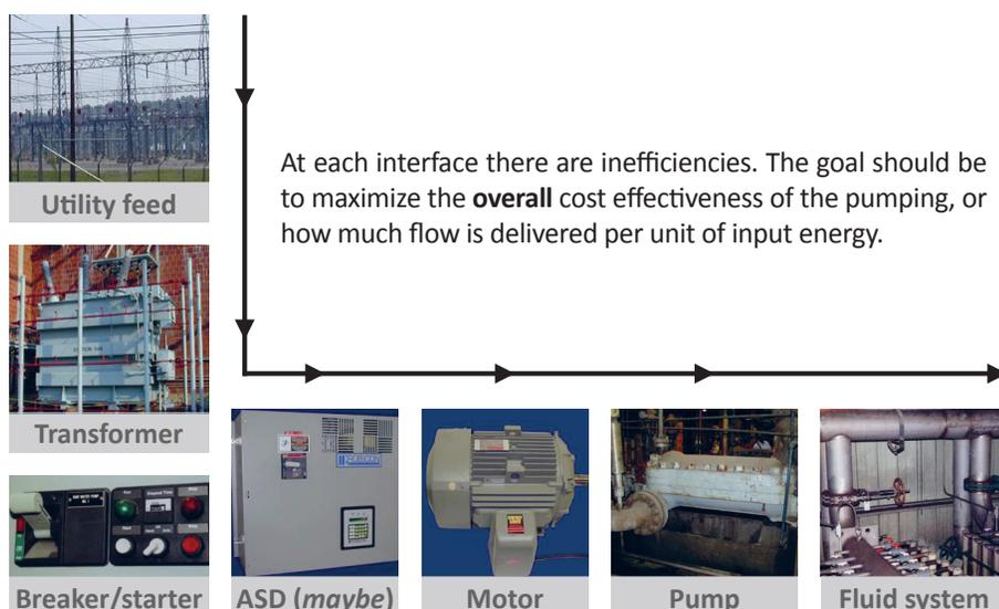
Fig. 2.1. System components
