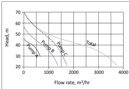
**Fig. 5.6.** Combined pump curve for pumps connected in parallel
