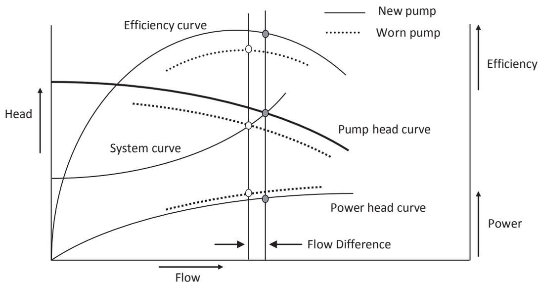
**Fig. 6.6.** Effect of worn pump on pump characteristics
