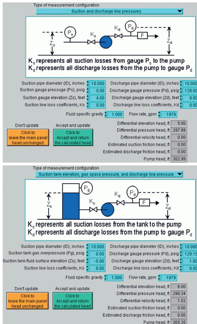
Fig. 12.17. Taps for Measuring Suction and Discharge Pressure
