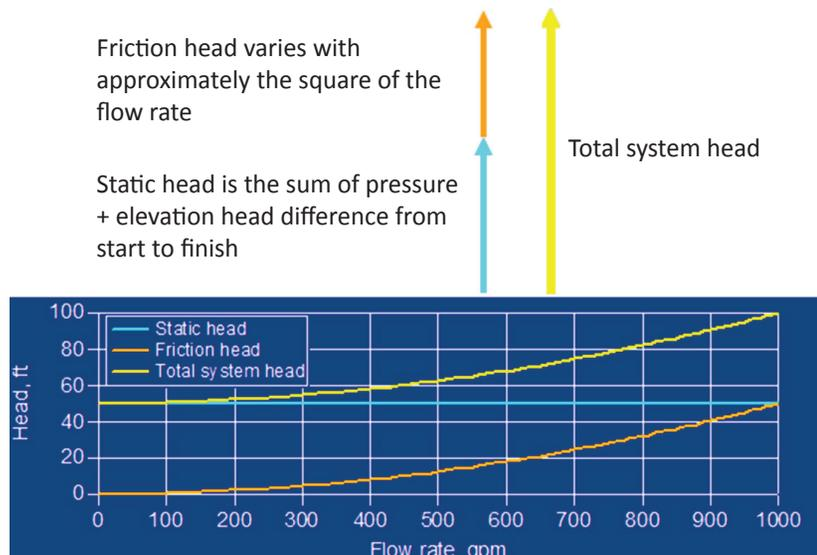
Fig. 12.8. Combination of Static Head and Friction Head
