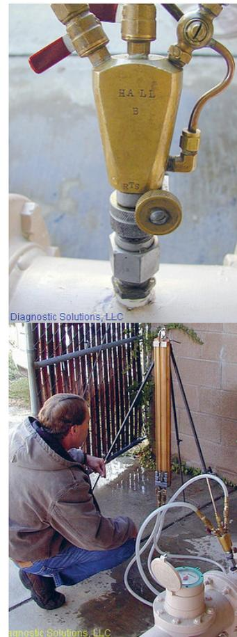
**Fig. 12.21.** Flow Reading with a Multi-port Pitot Tube
