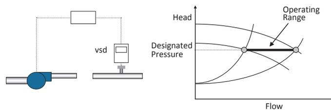
**Fig. 9.12.** Pressure controls with vsd equipped pump
