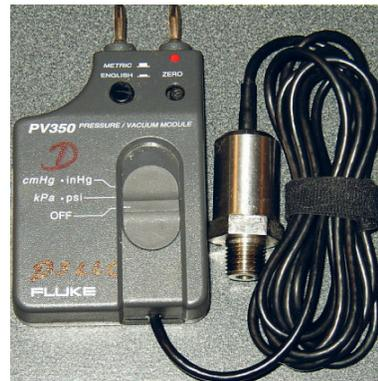
**Fig. 12.14.** Inaccurate Pressure Gauge and PV-350 Pressure Indicator
