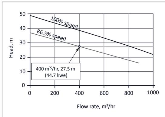
To develop 400 m<sup>3</sup>/hr in the all-static head system, the speed reduction needed to achieve 50% flow is even less, 86.5% of the original. The pump efficiency changes even more in this case. Figure 9.21.
