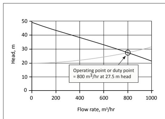
**Fig. 5.5.** System and pump curves with operating point
