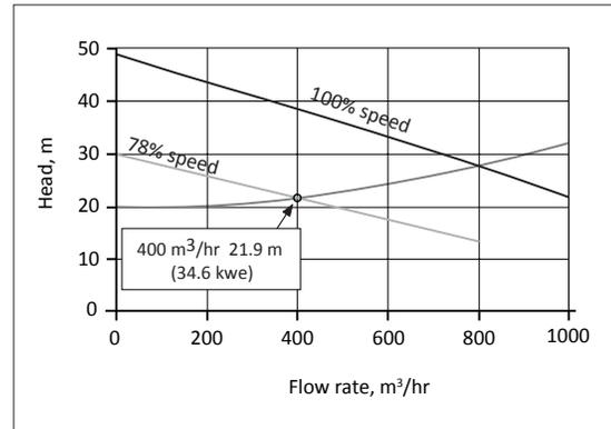
**Fig. 9.20.** Speed change in the mixed static/frictional system
