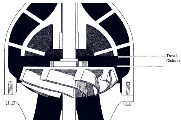
**Fig. 6.7.** Travel distance for a vertical turbine pump
