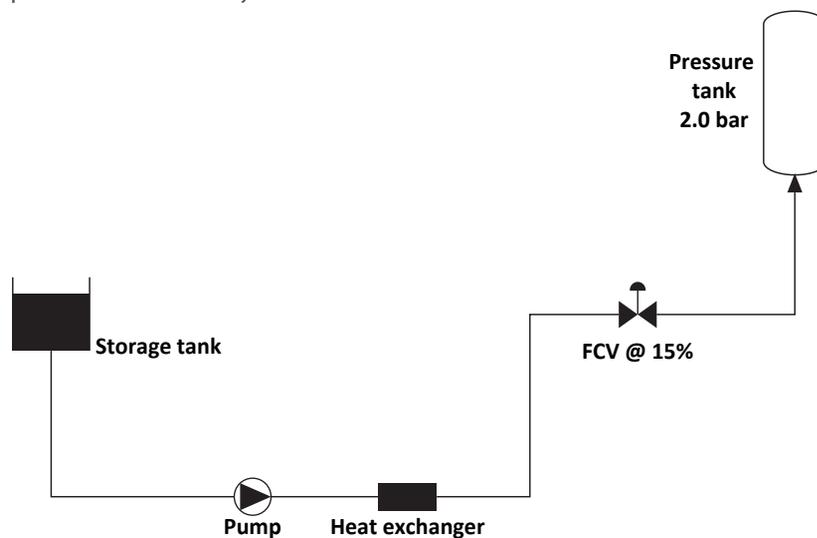
**Fig. 14.1.** Sketch of pumping system in which the control valve fails.
