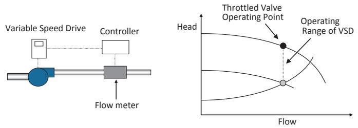
Fig. 9.13. Pressure controls with vsd equipped pump
