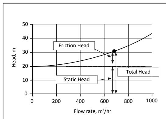
**Fig. 4.3.** System Curve Components
