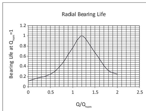
Fig. 6.4. Typical radial bearing life as a function of normalized flow rate
