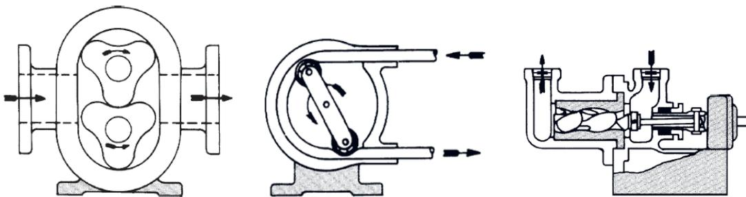
**Fig. 3.8.** Examples of Rotary Lobe, Tube and Screw Pumps
