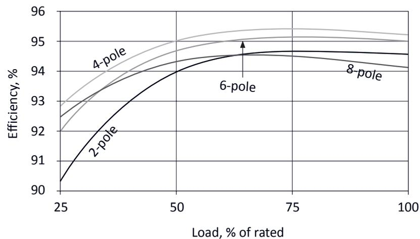
Fig. 8.3. Typical efficiencies for 60Hz, 75 kW motors
