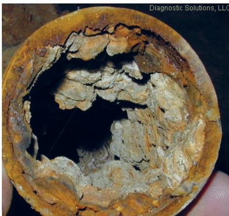
**Fig. 4.2.** Water distribution pipe with significant tuberculation (courtesy of Diagnostic Solutions)
