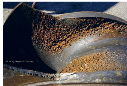
**Fig. 5.10.** Cavitation damage on an impeller
