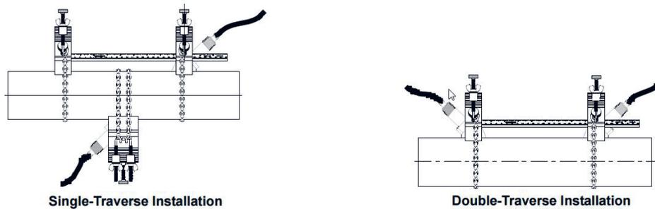
**Fig. 12.23.** Single and Double Traverse Methods
