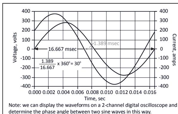
Fig. 12.26. Time Between Zero crossings of the Waveforms
