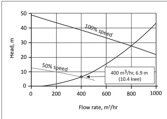
**Fig. 9.19.** Change in speed for the all-frictional system
