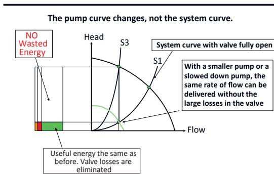
**Fig. 9.22.** This shows how the throttling losses and excessive losses in pump and motor are avoided when using a variable speed drive. It should be observed that this is the most favorable situation when there is no static head in the system.
