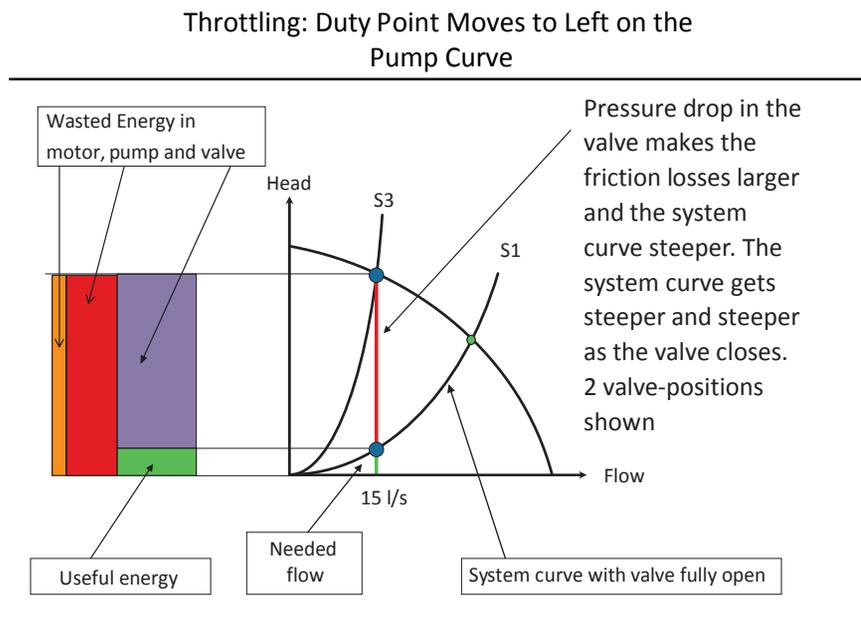
**Fig. 9.5.** The pump is further throttled and the operation point moves to the left. The pump efficiency has fallen even more and the losses in the valve have also increased. Only a small fraction of the energy supplied to the motor is used to move fluid.
