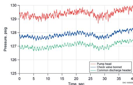
Fig. 12.6. Gauge Pressure Varies with Location and Time
