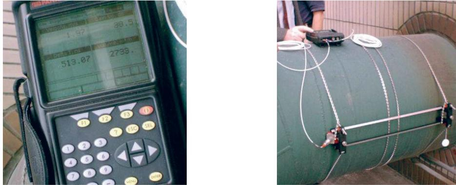
**Fig. 12.22.** Transit-time ultrasonic flow meter
