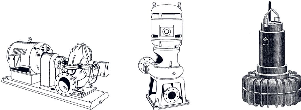
**Fig. 3.4.** Frame mounted and close coupled pumps
