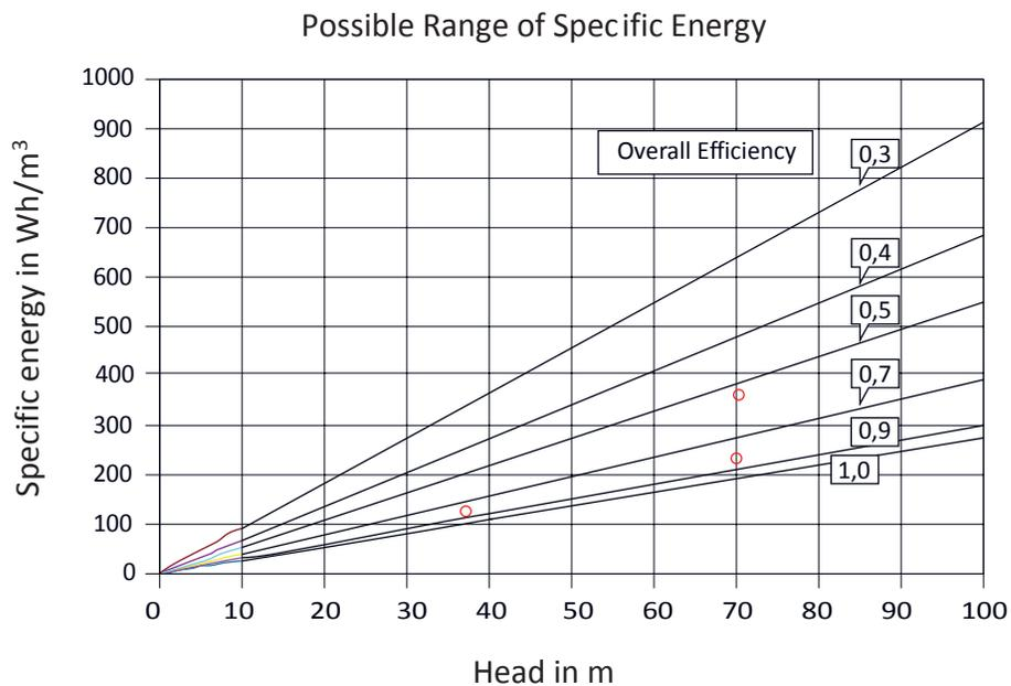
**Fig. 7.5.** Specific Energy Diagram with Three Operating Points.
