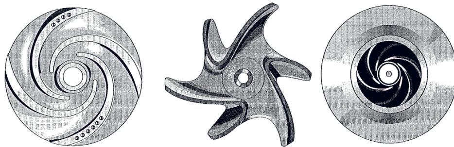
**Fig. 3.7.** Impeller types (semi-open, open and closed)
