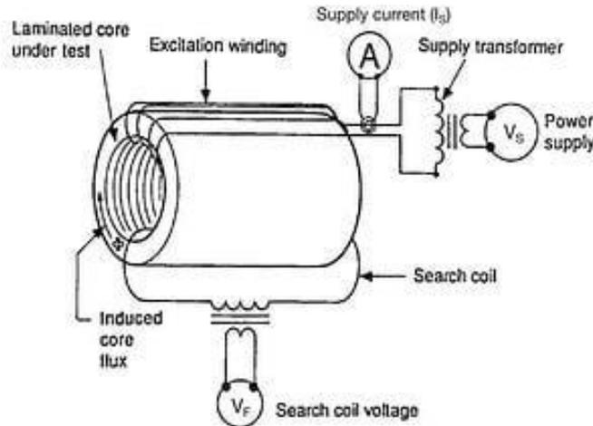
**Figure 64; Core Test Configuration**
