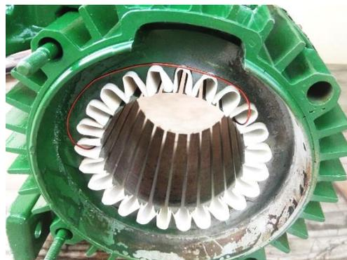
Figure 41, Completely Isolated Stators Slots
