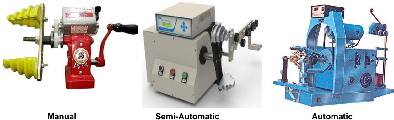
**Figure 42; Coil Winding Machines**
