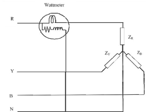
**Figure 61; Single Wattmeter Method of Power Measurement in 3-Phase Circuit**
