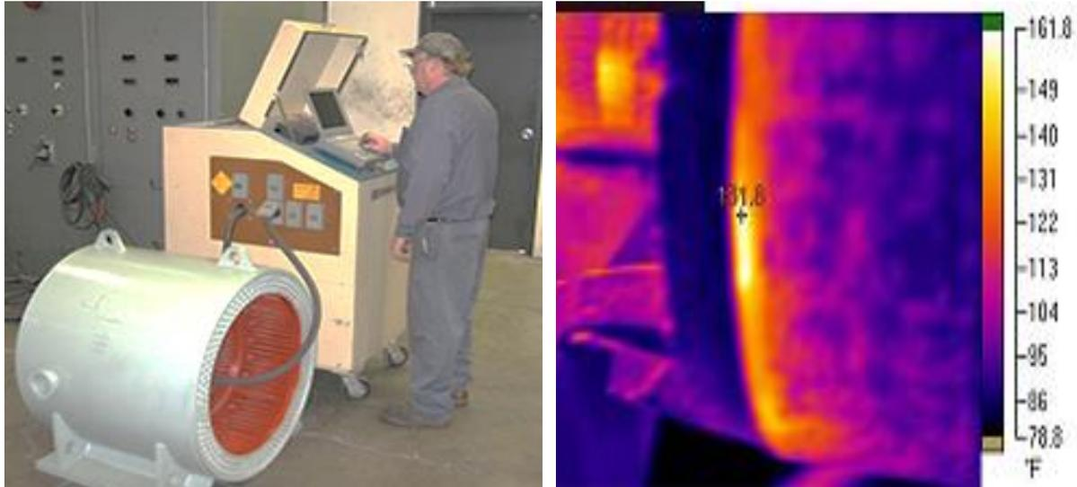
**Figure 66; Commercial core testers and Infrared core results**
