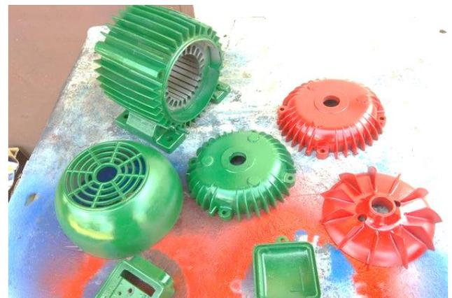
**Figure 39; Sandblasting and Painting the Stator**
