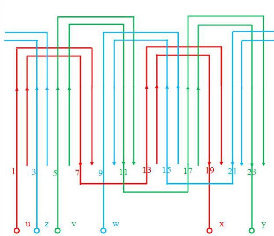
Figure 18; 3 Phase – 4 Poles - 24 Slots - Single Layer Concentric Winding – 50 Hz
