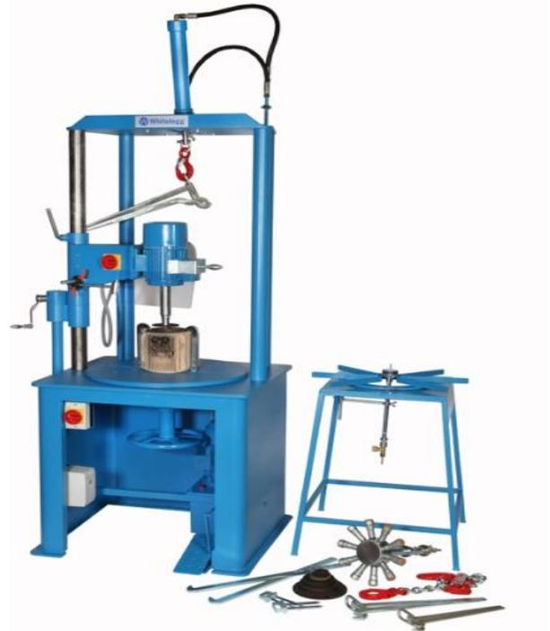
Hydraulic coil cut-off and extraction machine
