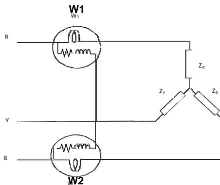
**Figure 62; Two Wattmeter Method of Power Measurement in 3-Phase Circuit**
