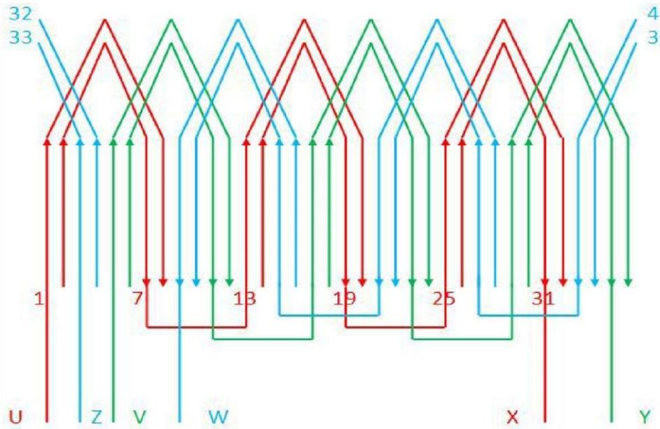
Figure 20; 3 Phase – 6 Poles - 36 Slots - Single Layer Concentric Winding – 50 Hz
