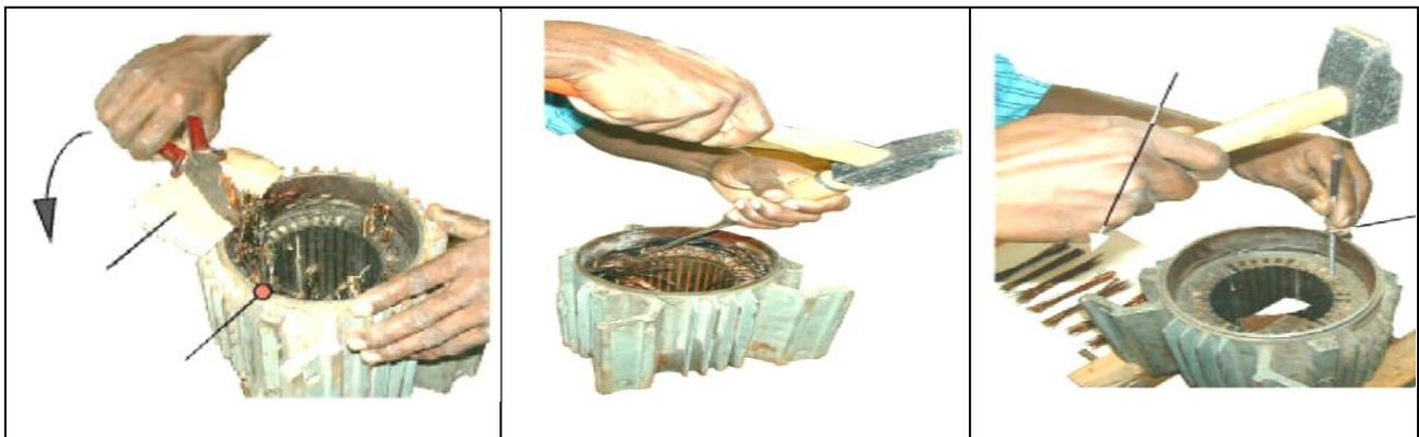
**Figure 34; Winding Cut-off Manually**
