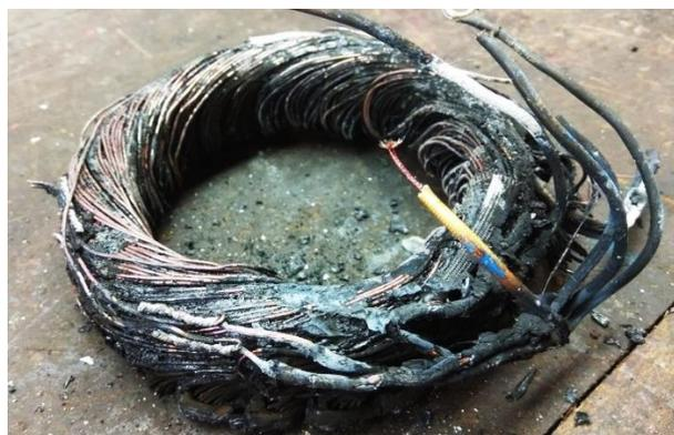
Figure 36; Burned Winding Head
