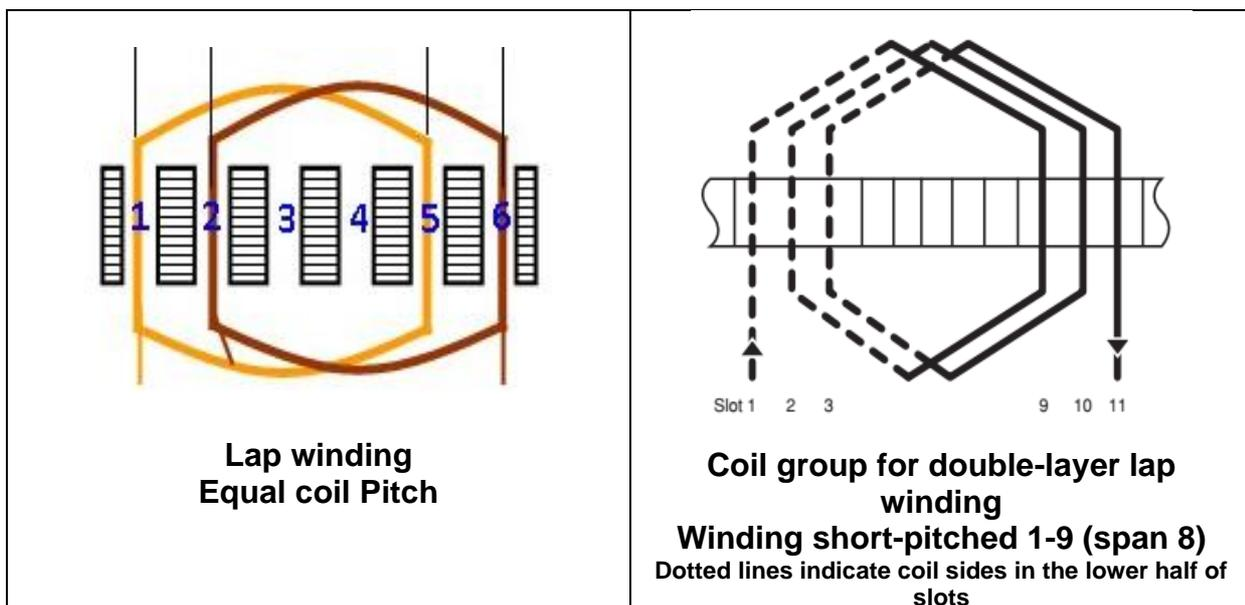
Figure 12; Lap Winding
