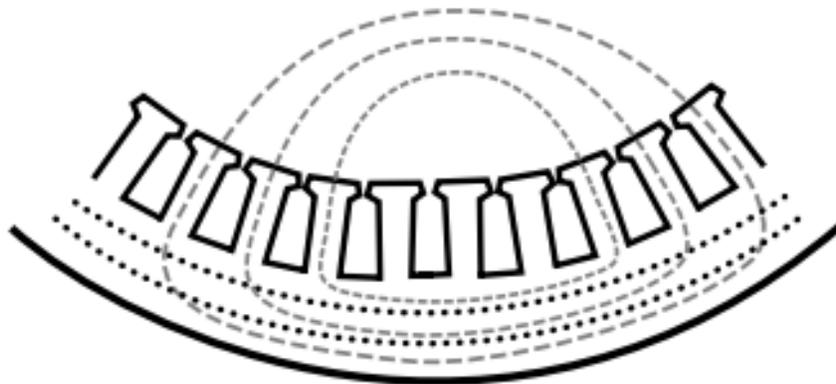
**Figure 65; Flux induced by the machine's winding when the rotor is removed**
