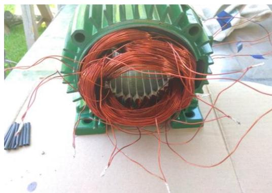
**Figure 45; Connecting Coils**
