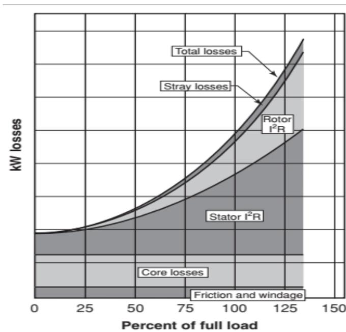
Figure 23; Different Losses Components as a Function of Motors' Loading
