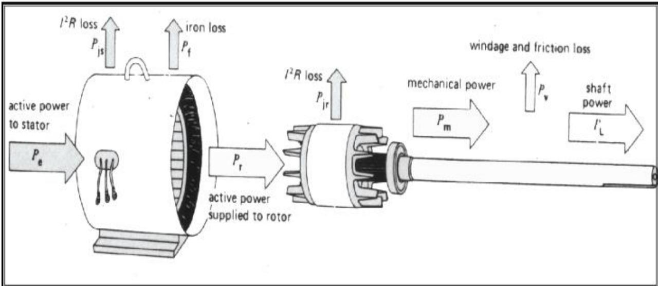
Figure 22; Schematic Diagram Showing Losses in Three-phase Induction Motors
