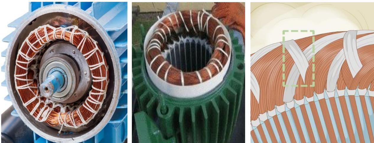
Figure 46; Lacing and Bracing Windings
