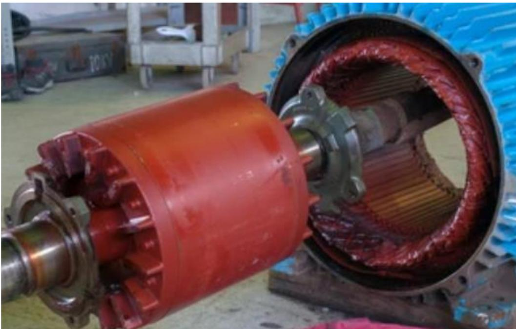
Figure 29; Remove Rotor from Stator
