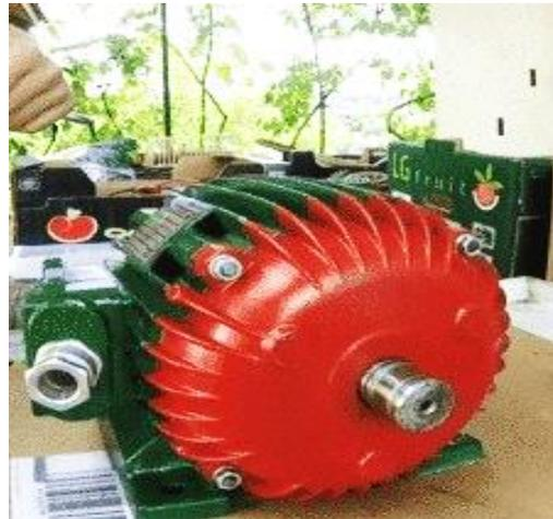
Figure 53; Reassemble Fan and Fan Cover
