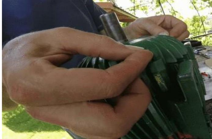
Figure 51; Putting the Rotor into Stator
