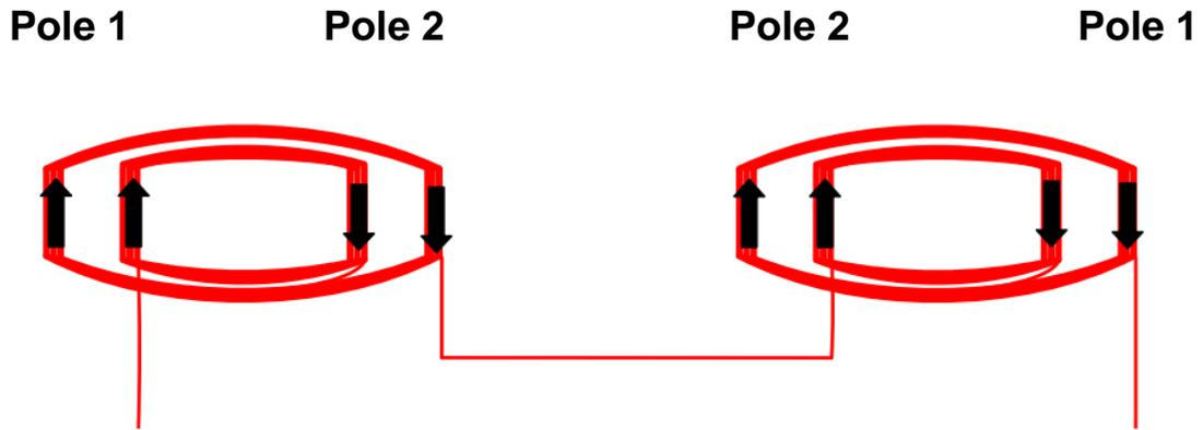
**Figure 15; Half Coil Winding**
