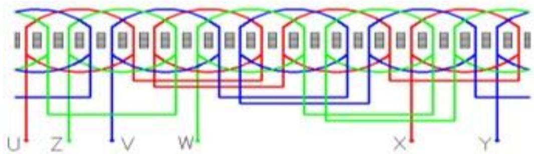
Figure 19; 3 Phase – 4 Pols - 24 Slots - Single Layer Lap, Winding – 50 Hz
