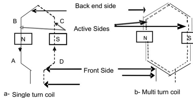
**Figure 7; Winding Coil Representation**
