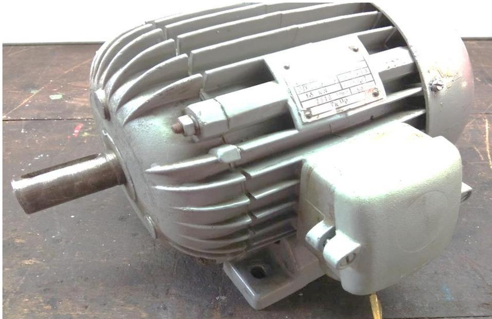
**Figure 1; Three Phase Squirrel Cage Induction Motor**
