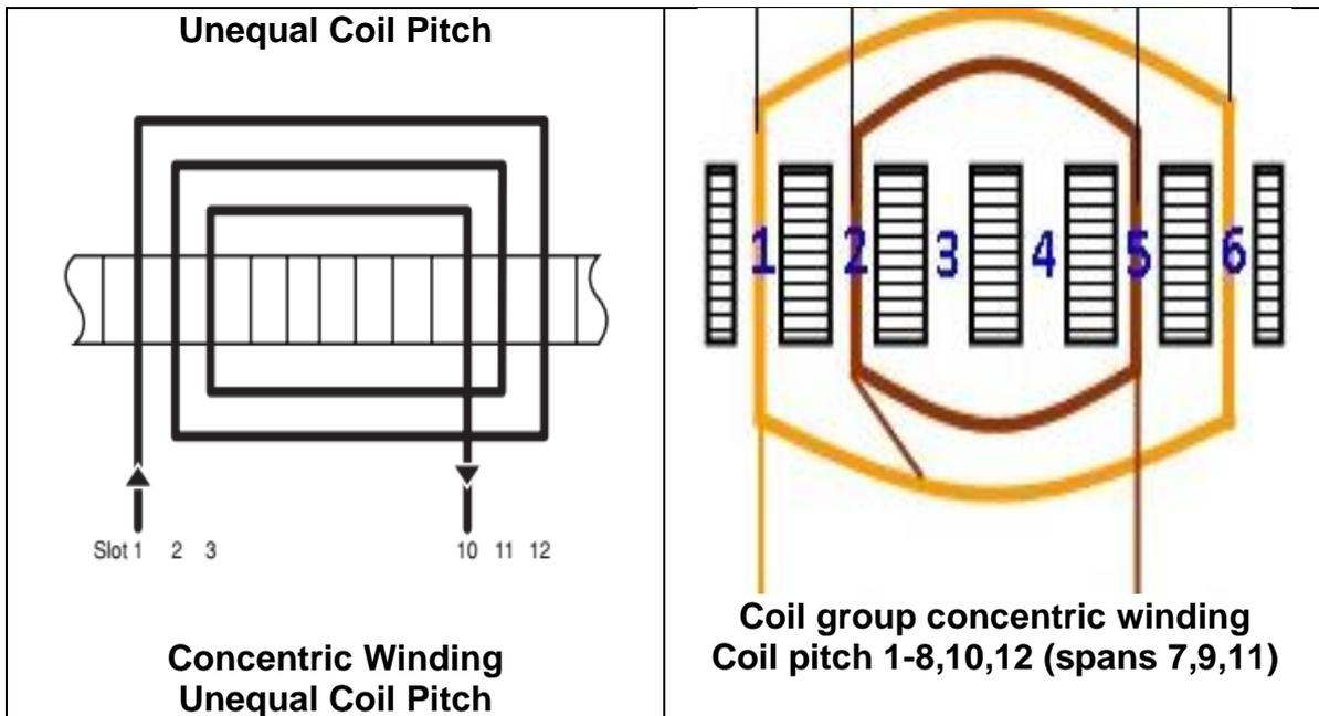
Figure 13; Concentric Winding
