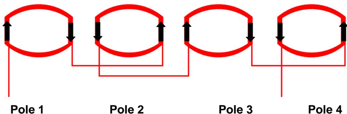
Figure 14; Whole Coil Winding
