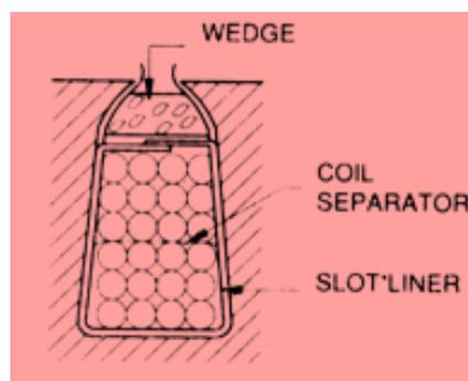
**Figure 5; Slot Insulation**
