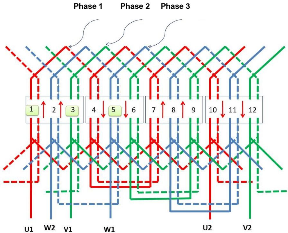
Figure 21; 3 Phase – 4 Poles - 24 Slots - Double Layer – 50 Hz
