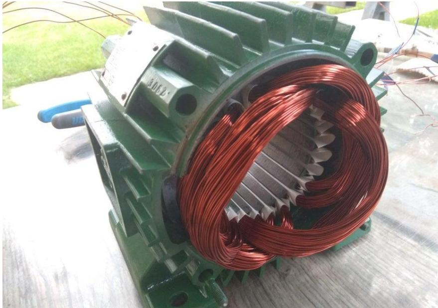
*Figure 6; Rewinding the Motor*
