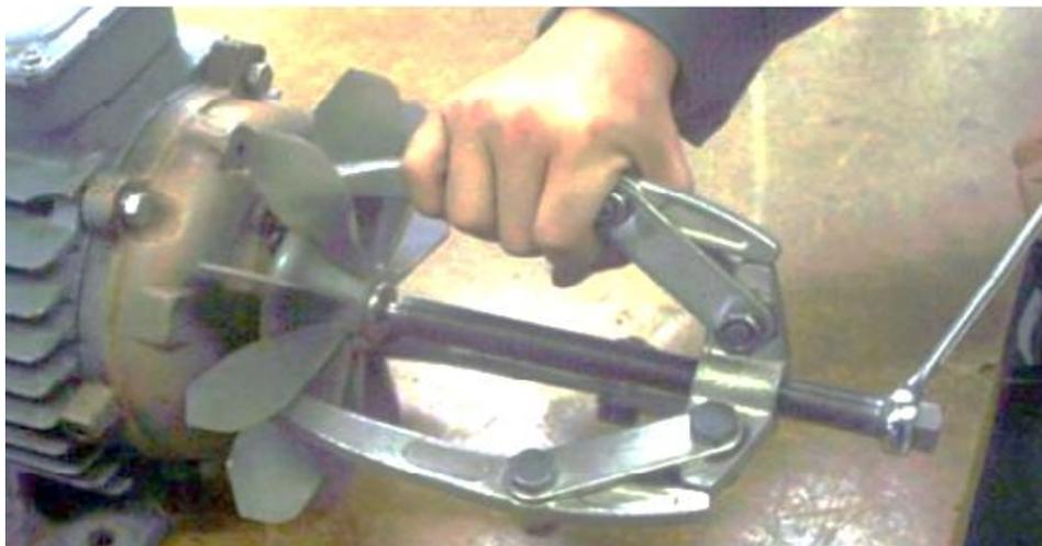
Figure 27; Removing the Fan and the Second Cover
