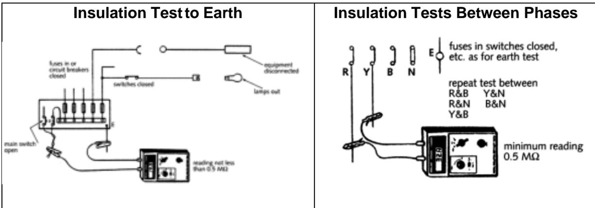
Figure 60; Samples of Insulation Testing
