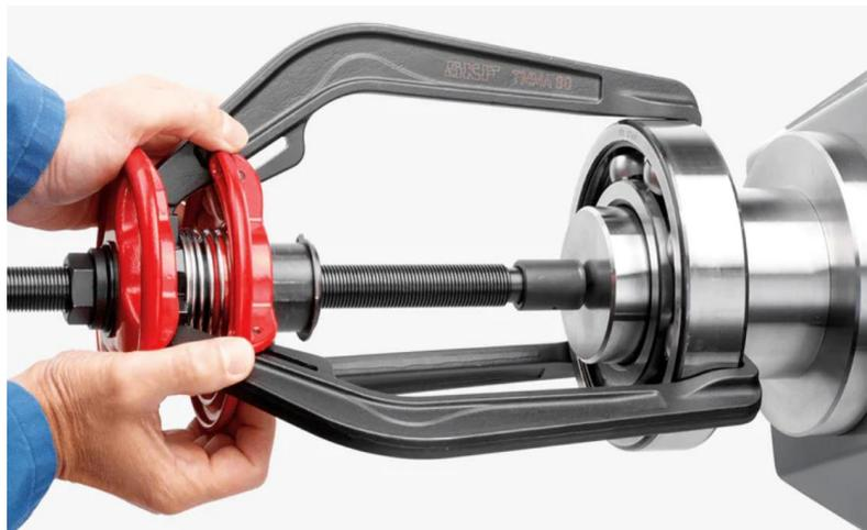
Figure 28; Removing the Bearings
