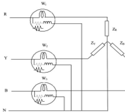
**Figure 63; Three Wattmeter Method of Power Measurement in 3-Phase Circuit**
