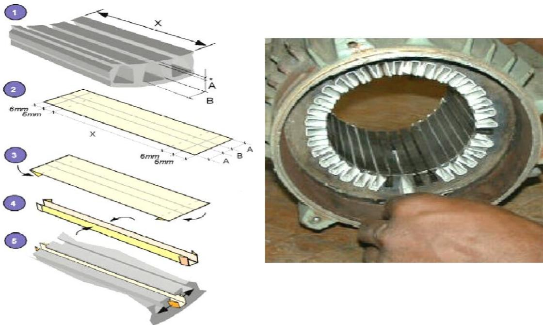
Figure 40, Isolating Stators Slots
