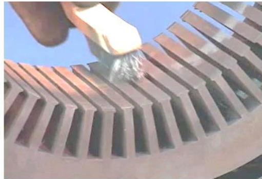
**Figure 38; Cleaning the Stator Core**
