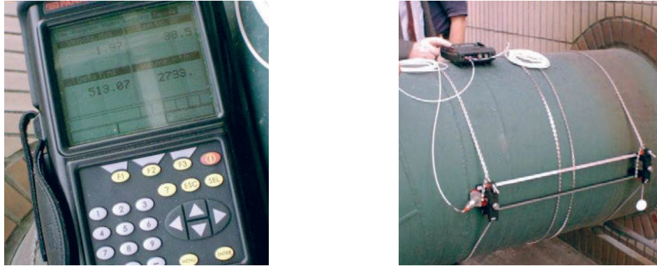
Fig. 12.22. Transit-time ultrasonic flow meter
