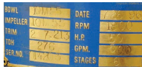
Fig. 12.1. Motor and Pump Nameplate Data
