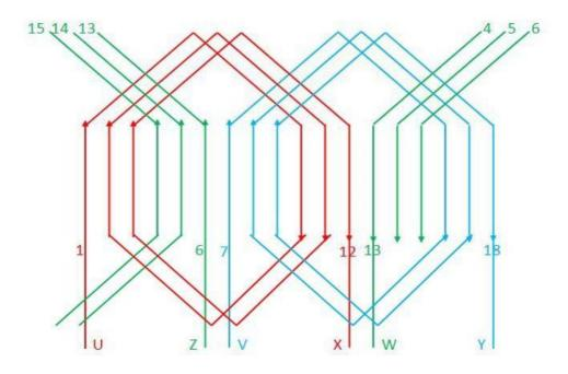
Figure 16; Figure 16; 3 Phase – 2 Pols - 18 slots - Single layer – 50 Hz
