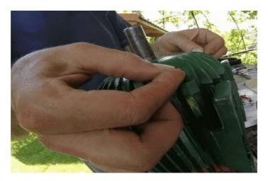
Figure 51; Putting the Rotor into Stator
