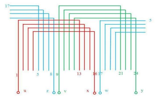
Figure 17; 3 Phase – 2 Pols - 24 slots - single layer – 50 Hz
