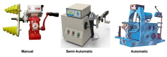
Figure 42; Coil Winding Machines
