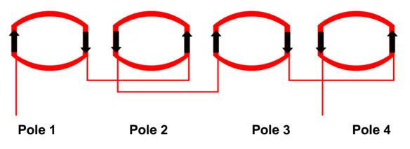
Figure 14; Whole Coil Winding
