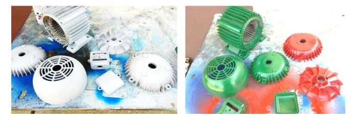
Figure 39; Sandblasting and Painting the Stator
