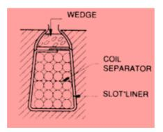
Figure 5; Slot Insulation
