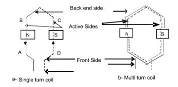
Figure 7; Winding Coil Representation
