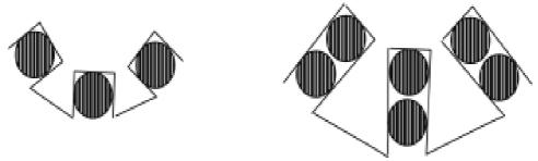
Figure 10; Single Layer and Double Layer Winding
