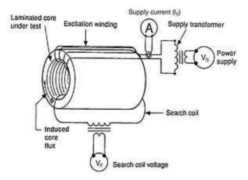
Figure 64; Core Test Configuration
