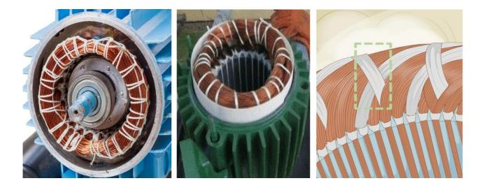
Figure 46; Lacing and Bracing Windings
