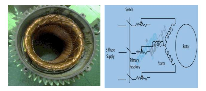
Figure 3; Stator of 3-phase Induction Motor
