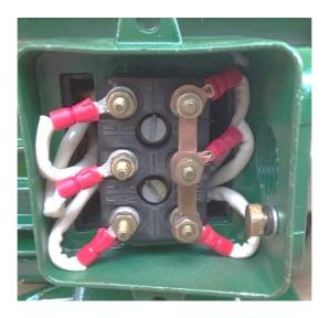
Figure 52; Connect End of Coils to Clips in the Terminal Box
