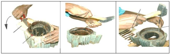
Figure 34; Winding Cut-off Manually
