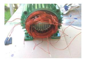
Figure 45; Connecting Coils
