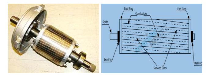
Figure 2; Rotor of 3-phase Induction Motor
