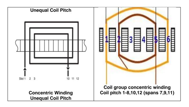
Figure 13; Concentric Winding
