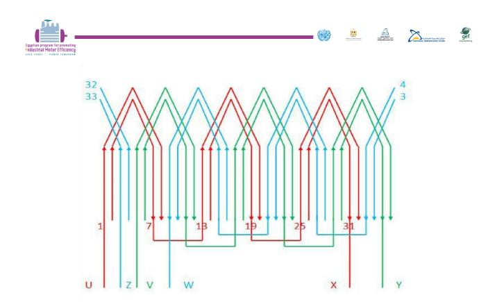
Figure 20; 3 Phase – 6 Pols - 36 Slots - Single Layer Concentric Winding – 50 Hz
