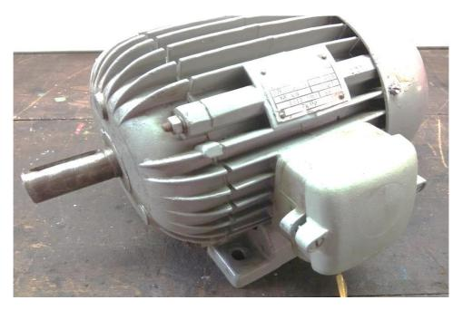
Figure 1; Three Phase Squirrel Cage Induction Motor
