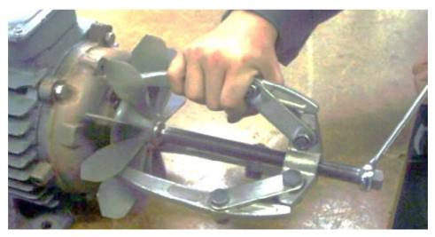
Figure 27; Removing the Fan and the Second Cover
