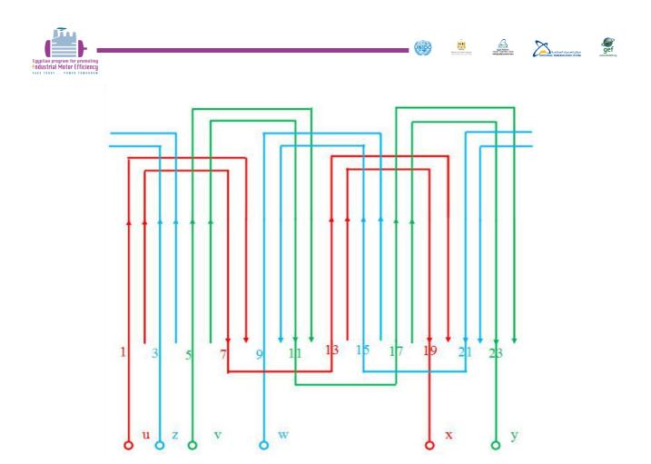
Figure 18; 3 Phase – 4 Pols - 24 Slots - Single Layer Concentric Winding – 50 Hz
