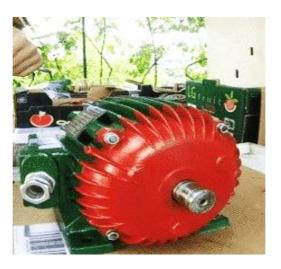
Figure 53; Reassemble Fan and Fan Cover
