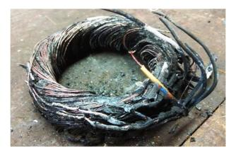
Figure 36; Burned Winding Head
