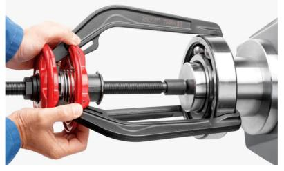
Figure 28; Removing the Bearings
