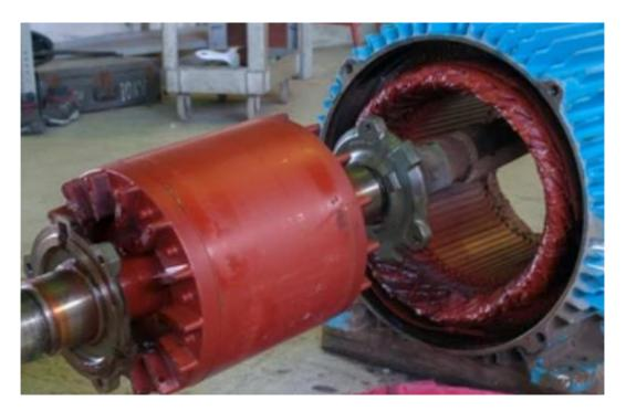
Figure 29; Remove Rotor from Stator
