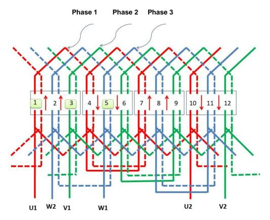
Figure 21; 3 Phase – 4 Pols - 24 Slots - Double Layer – 50 Hz
