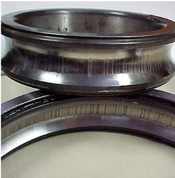
Figure 9 Example of Motor Shaft Voltage and Bearing Current Damage [7], Source: Renown Electric
