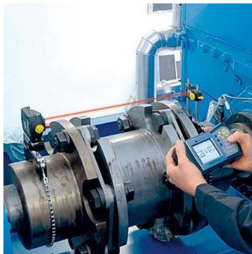
Figure 71 Modern laser alignment equipment (directindustry.com)
